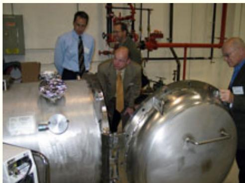
LCFOA members inspect a horizontal test cryostat at an ILC test area.
