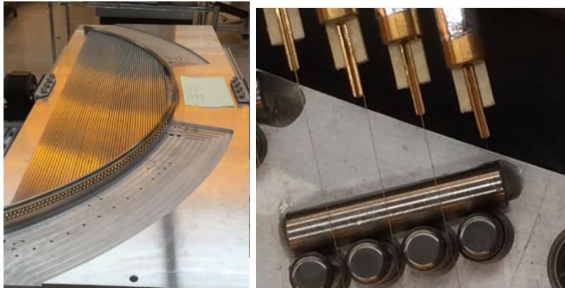
Figure 1: The first Mu2e tracker prototype panel. The left figure shows 96-straw panel. The right figure is a close-up of the straw terminations and the dowel pins used for positioning the sense wires.
