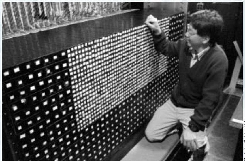
Bob Hsiung inspects the calorimeter at the heart of the KTeV detector during installation in the summer of 1996.
