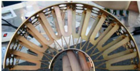
Fluorocarbon will flow through these U-shaped channels to keep CMS electronics operating at -10 degrees Celsius. "Without cooling, the temperature of the electronics mounted directly on the silicon pixels could be high enough to prevent normal operation," said physicist Bruno Gobbi, who helped work on sketches for the design.
