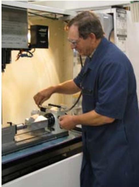
Harry Parkhurst uses machines to translate engineers' plans into reality. The platform above will oscillate around a drill (top left), boring holes with perfect angles and dimensions.
