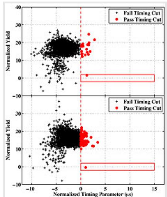
In these figures, the dotted red line divides events into those determined not to be WIMPs based on the relative timing of the heat to charge signals (left side) and those that could potentially be WIMPs based on that parameter (right side). The solid red box delineates the area of the graph in which WIMPs should occur based on both timing and the heat to charge ratio. Two events in separate detectors demonstrated the characteristics scientists predicted a WIMP would have.
