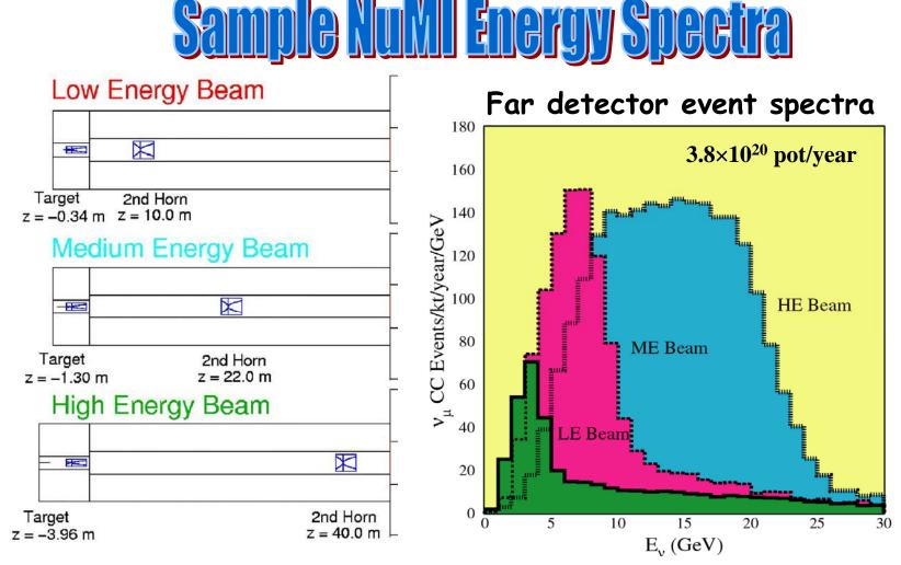
• Fully optimized spectra for each energy are obtained by moving the target and the 2<sup>nd</sup> horn
