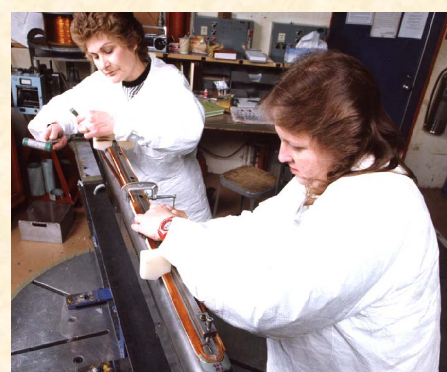
Winding LBQ coils.
