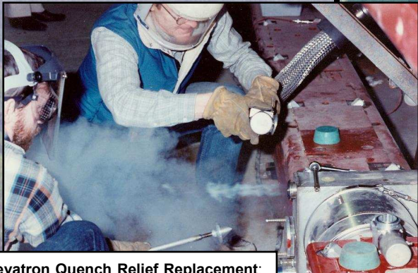
Tevatron Quench Relief Replacement: Ken Olesen (left) and Jay Theilacker replacing a relief valve on a Tevatron dipole at 20 K.
