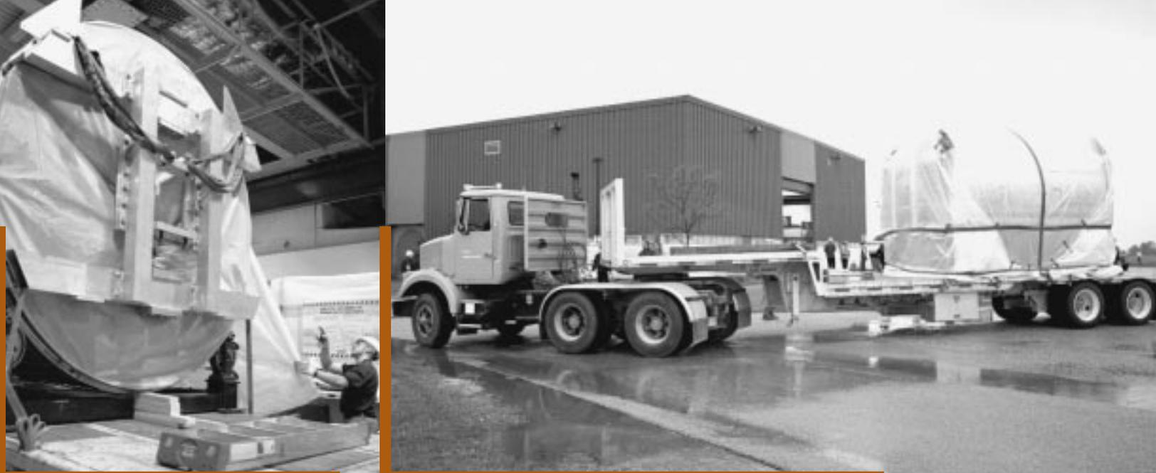
The Central Outer Tracker is loaded onto a special low-riding, air-suspended flatbed truck from its assembly site in Industrial Center Building 4 (left), covered to protect it from the elements (center), and wheeled outside to prepare for its journey across D Road to the CDF Assembly Hall (right).
