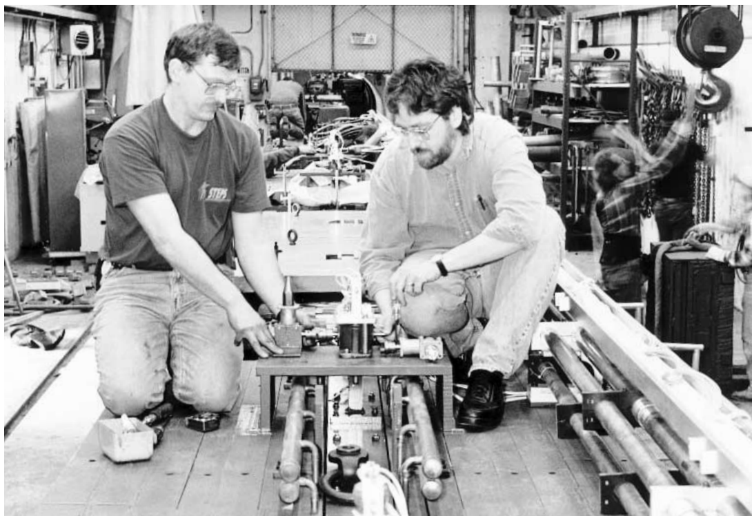
John Voirin and Bob Bernstein adjust supports for the proton dump of the Sign-Selected Quad Train, E815's beamline.
