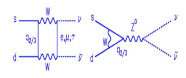
One of the Golden Modes for study of the CKM matrix and CP violation. The rate can be calculated precisely (~8% now→~5% future) from the fundamental SM parameters, and hence any deviation in the measured rate will be a clear signal for new physics. □ 0.4
