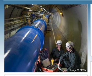
The LHC is the largest, most complex and most powerful particle collider ever built. It will operate at CERN near Geneva, Switzerland in a 17-mile circular tunnel about 300 feet underground. The LHC will create 600 million proton-proton collisions per second at an energy of 14 trillion electron volts, using beams of protons seven times more energetic and about 30 times more intense than those ever before produced.
