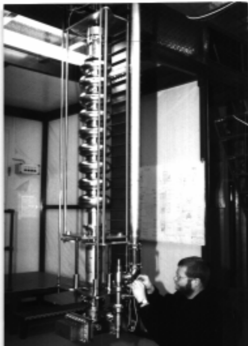
Figure 5: One of the TESLA Niobium resonators being prepared for CW-RF test in the vertical test stand.
